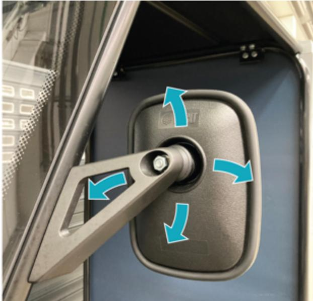
*Fig. 13 Adjusting the mirror*
